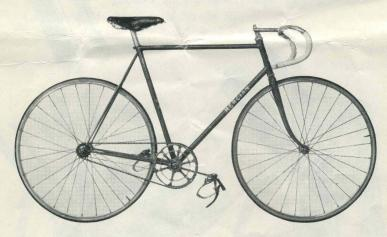
In Pursuit trim, total weight of machine using steel stem, steel cranks, 28 spoke sprints and silk O's, can be got down to 16 lb. 13 ozs.
